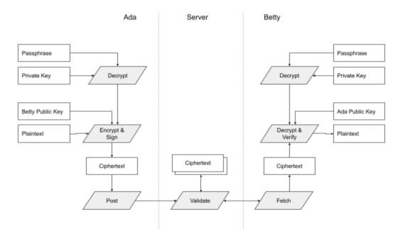
Fig. Encryption and decryption cycle in passbolt
