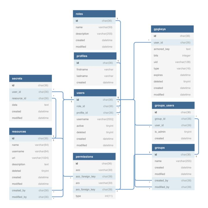
Fig. passbolt core data model
